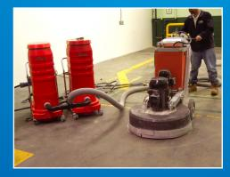
VACUUM ASSIST TOOLS FOR SILICA DUST REMOVAL
